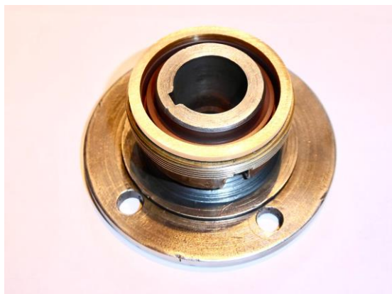
Showing seal position on flange boss
