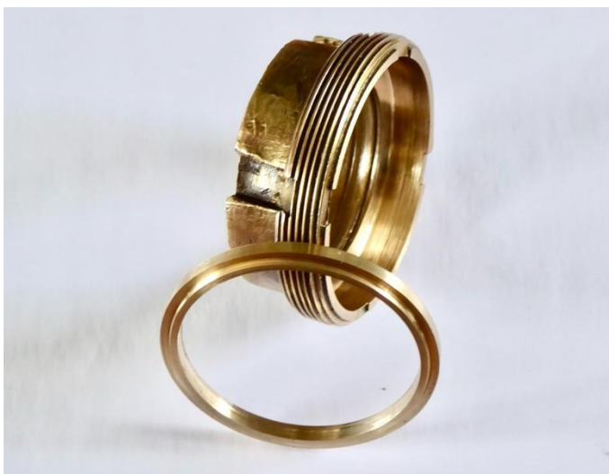
Machined Retainer & New Back Ring
