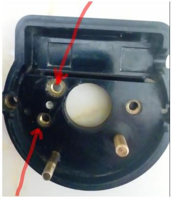
The two arrows indicate the earth return points for the Condenser and C/B, also they indicate where a temporary earth feed can be attached.
