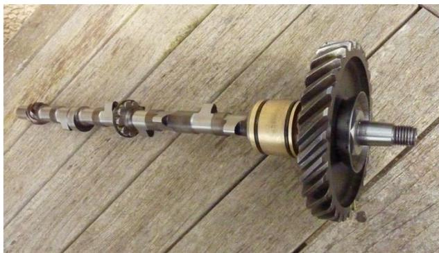
Camshaft assembly ready for insertion
