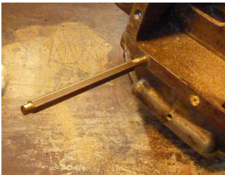
Installing a brass bush prior to cutting-off flush
