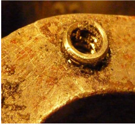
One or two raised 'Helicoils'
