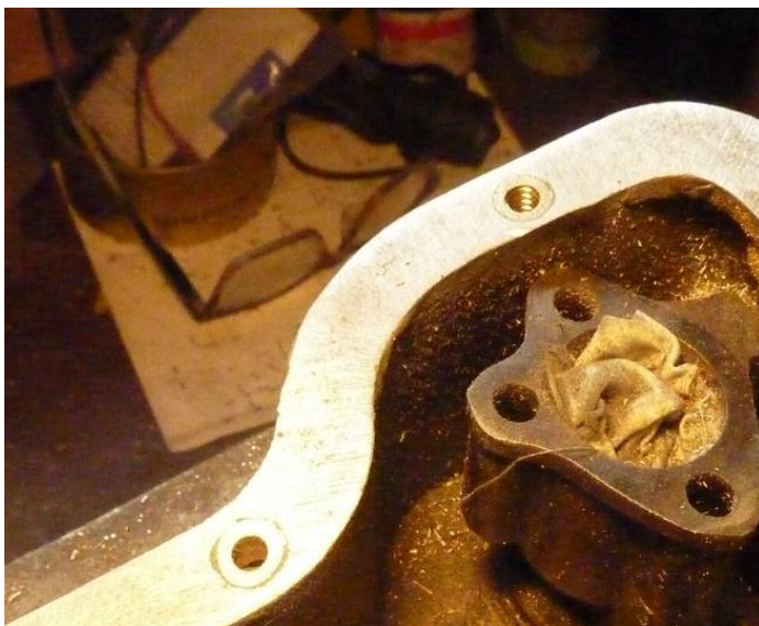
Brass inserts complete and threaded ¼" BSW
