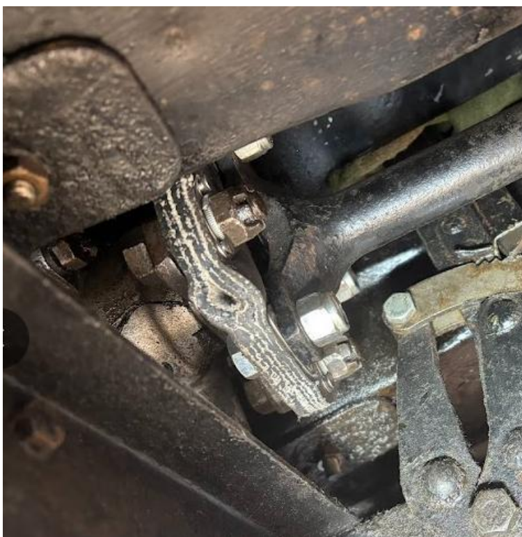
Failed fabric coupling
