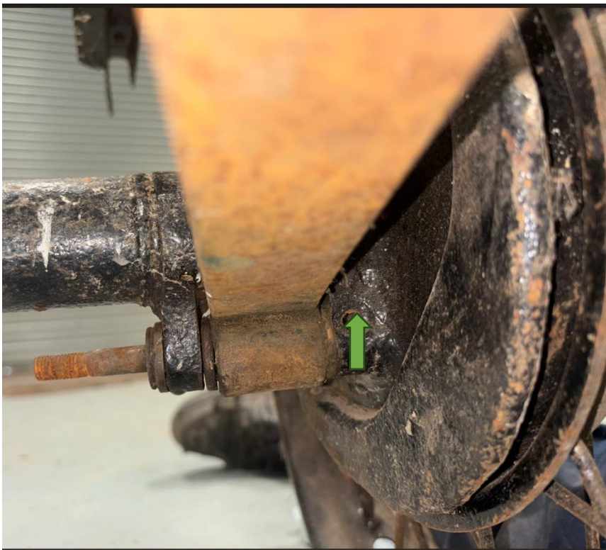
View from front left side of rear axle. Note hole for cotter pin (green arrow) and rest of spring pin sticking out to left for attachment of damper
